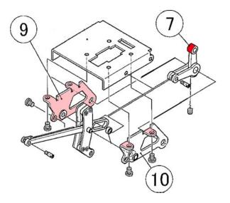
3) As shown by the left diagram it is necessary to file off the top of 2-7 as marked in red, so that it does not hit the 2-8 bottom side.
