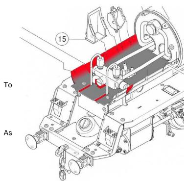
When you assemble the Smoke box 12- 9 to the Boiler cover, it is necessary to loose the screws M2-4 of the Back head 8-6. Then after fixing the Smoke box cover you can tight the Back head screws. Do not try to squeeze the Smoke box cover and fix in to the Boiler case.
