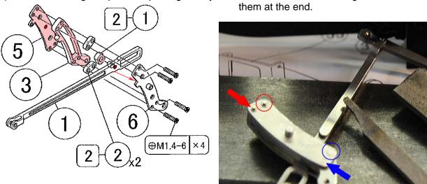
After finishing the Section 6 and 7 valve settings and when you set the Reverser lever to the neutral position, all the rods and wheels must be same as per illustration below.
