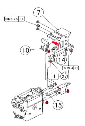
1) The parts marked in red 4-10 and 4-7 are LW parts, may be it is necessary to file off a bit in the area marked in red. Also may be it is necessary to file off the top of Cross head and to make it thinner.
