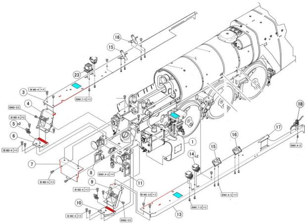
**Section 11 -** When you want to fix the running boards correctly, do not file off the places marked in Cyan color. Try to trim the positions marked in Red to file off and fix the running Board
