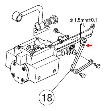
4) Part 2-18 - Please make the hole bigger, marked in red to make it to 1.65mm size and at present it is 1.5mm.
