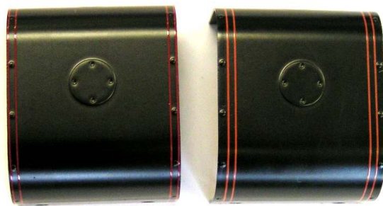
The correct cylinder shrouds for black livery (left) and for green livery (right).
